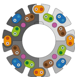
SGH 16.1 female Wiring diagram
