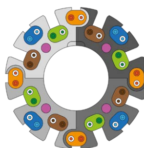
SGH 16.1 male Wiring diagram
