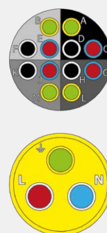
Central insert male Wiring diagram SGH 8.1 | SGH 16.1
