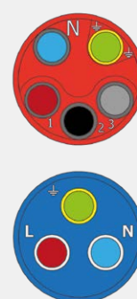
Central insert male Wiring diagram SGH 8.1 | SGH 16.1
